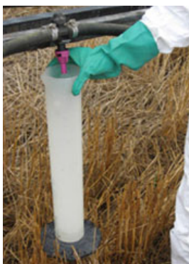
Figure 2. In a stationary position and with proper boom pressure, measure the output over the same time period used for the run. The number of ounces collected is equal to the gallons per acre.
